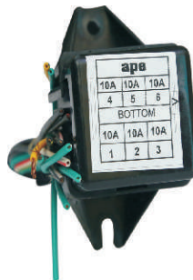
FUSE BOX APE (3 WHEELER)
